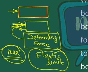
When external force is applied on a body it's shape or size changes ie the body be comes deformed when this force is removed the body again comes to it's original state. This property of the body is called elasticity.
