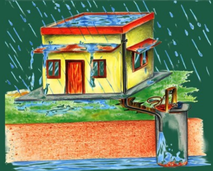
(b) Recharge Through Abandoned Dugwell
