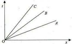
The figure shown above gives the time (t) versus position (x) graphs of three objects A, B and C. Which one of the following is the correct relation between their speeds  $V_A$ ,  $V_B$  and  $V_C$ , respectively at any instant (t > 0)?
