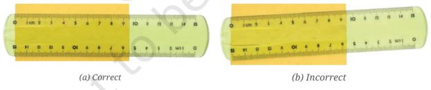
Fig. 5.4: Method of placing the scale
