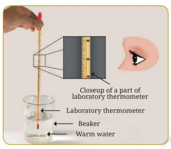
Fig.7.4: Measuring temperature of warm water
