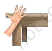
Fig. 5.1: Use of handspan for measuring
