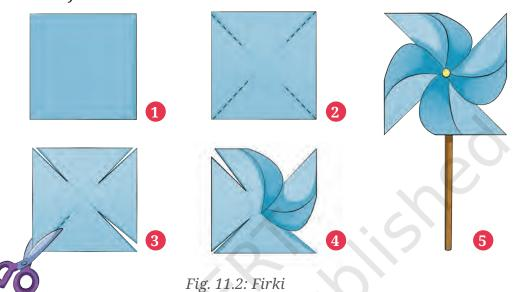
Now, you can hold the *firki* in your hand and run. You can also blow air on it. What do you observe? Does the *firki* rotate? When you move it a little back and forth, the *firki* rotates. What makes a *firki* rotate? It is the wind that makes a *firki* rotate.
