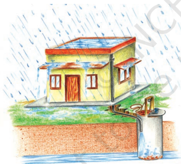
(b) Recharge through Abandoned Dugwell
