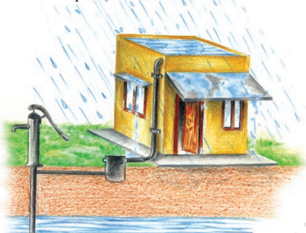
(a) Recharge through Hand Pump
