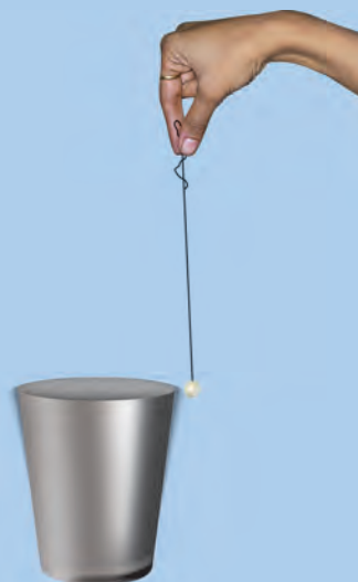
Fig. 10.17 : Thermocol ball touching the vibrating glass tumbler
