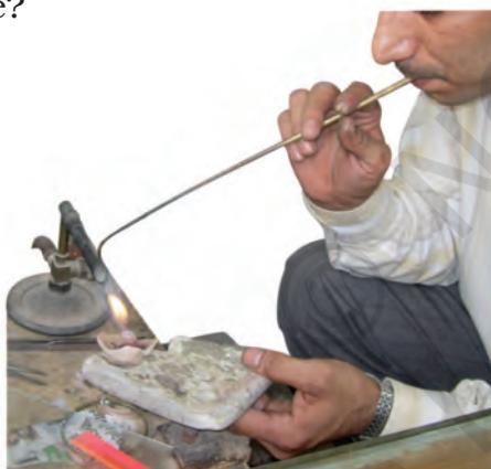
Fig. 4.14 : Goldsmith blowing through a metallic pipe
